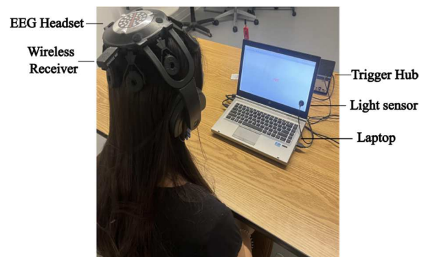
Figure 1. A participant completing the stimulus paradigm on a laptop while seated at a table. The light sensor connected to the Trigger Hub marks the onset of the Stroop stimuli. The wireless receiver transmits stimuli from the Trigger Hub to synchronize it to the EEG signal.
